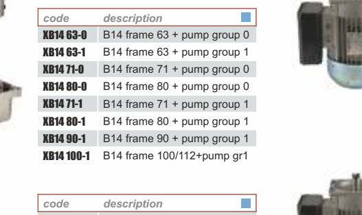
Note: DC motors and AC integral motors are directly mounted on the central manifold without adaptor flanges. Mounting kits are needed only to mount standard IEC B14 (international) or Nema (American) motors.
